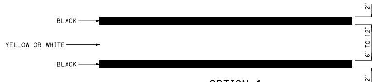
OPTION 1 TYPICAL LANE LINE OR RIGHT EDGE LINE CONTRAST DETAIL
